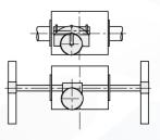
ARG: Supplied with worm drive shaft for remote adjustment from either end (to be specified). Also available with adjustment control (X).
