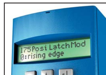
The POSILatch function uses external signals and evaluates them as measure- ment function. POSITatch can replace a separate PLC measuring system
