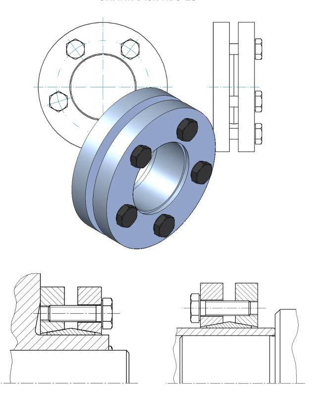
**KBS 19 External Clamping Set** is a friction detachable shaft-hub connection for cylindrical shafts and bores without keyway.
