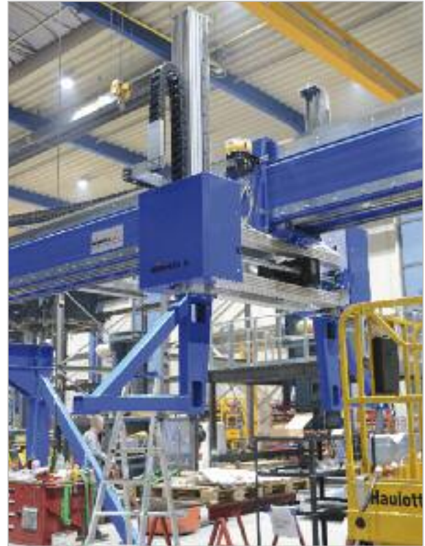
Examples of DLE linear axis
