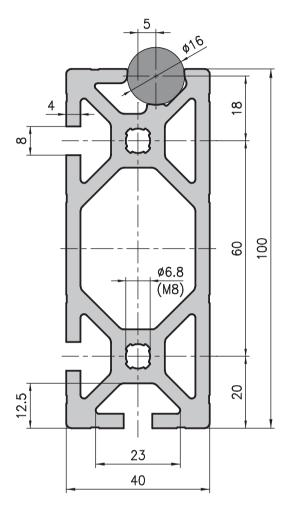
the front face in the holes  $\varnothing$  6.8 with a M8 thread.
