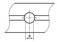
That drill, allows a connection for a parallel connector at any position at the extrusion.
