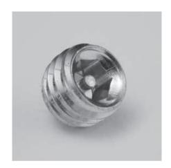
Special PVS® screw Safe M12x12 for safety constructions which must not be easy to dismantle by unauthorised persons. A pin inhibits access to the screw so that it cannot be unscrewed using a commercially available Allen key.
