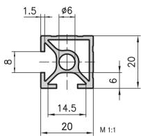
Helicoil inserts (DIN 8140) can be used for all extrusions with a core hole of  $\emptyset$  6 See machining code H3/H4.
