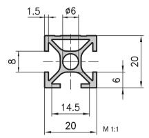
The 20x20 and 20x40 extrusions are also suitable as a support or reinforcement extrusion behind panels, which is in combination with the base 30 extrusion with panel slots (see sketch).
