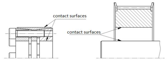
Image 3) cleaning the contact surfaces
