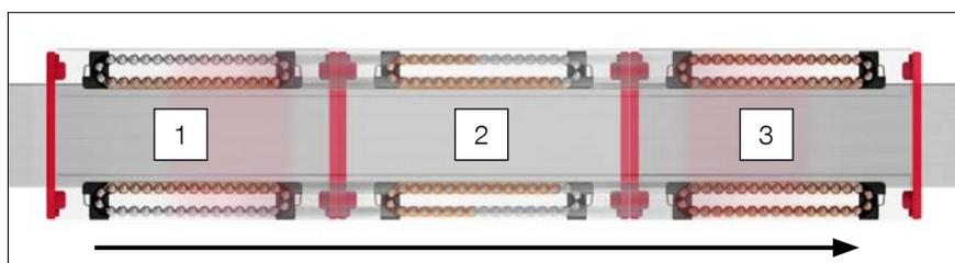
A short stroke is when the stroke of the carriage corresponds to less than twice its length. This can lead to damage, particularly in the redirection unit. Regular lubricating strokes along the entire stroke length at a minimum of twice the length of the carriage ensure better lubricant distribution, protecting the guideway from premature wear.
