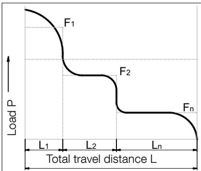
The loads ( $F$ ) acting on a linear guideway system are subject to frequent fluctuations during operation. This set of circumstances should be taken into account when calculating service life. The varying load absorption of the guideway at varying operating conditions during the travel distance is described as being the dynamic equivalent load  $P$ .
