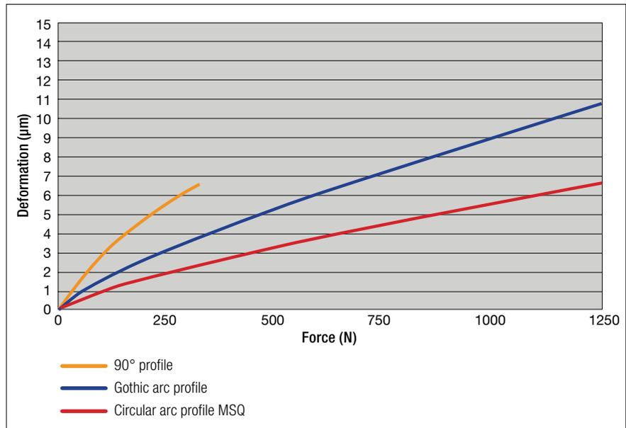
Comparison of the rigidity of structurally identical MINISLIDE size 9-80.66 with different contouring of the guideway tracks. The circular arc profile of MSQ results in the lowest deformation and therefore the highest rigidity
