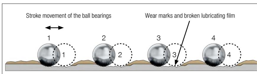
The stroke length of the guideway is so low that the rolling elements cannot pass the position of the next rolling element. As a result, local wear marks form on the tracks. Overstraining the tracks with short strokes leads to material damage which inevitably leads to the loss of preload. The accuracy of the guideway can consequently be reduced which can lead to premature failure.
