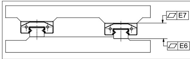
For the flatness of the guideway surface E<sub>6</sub> across the entire length, referring to the values for running accuracy for the appropriate accuracy class as described in chapter 7.2.4 is recommended.
