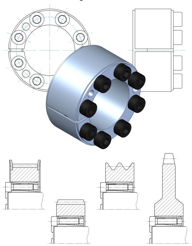
**KBS 52 Locking Device** is a frictionally engaged detachable shaft-hub connection for cylindrical shafts and bores without keyway.
